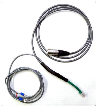
My interface cable. RJ45 to speaker connection spade lugs and XLR connector to Max processor
