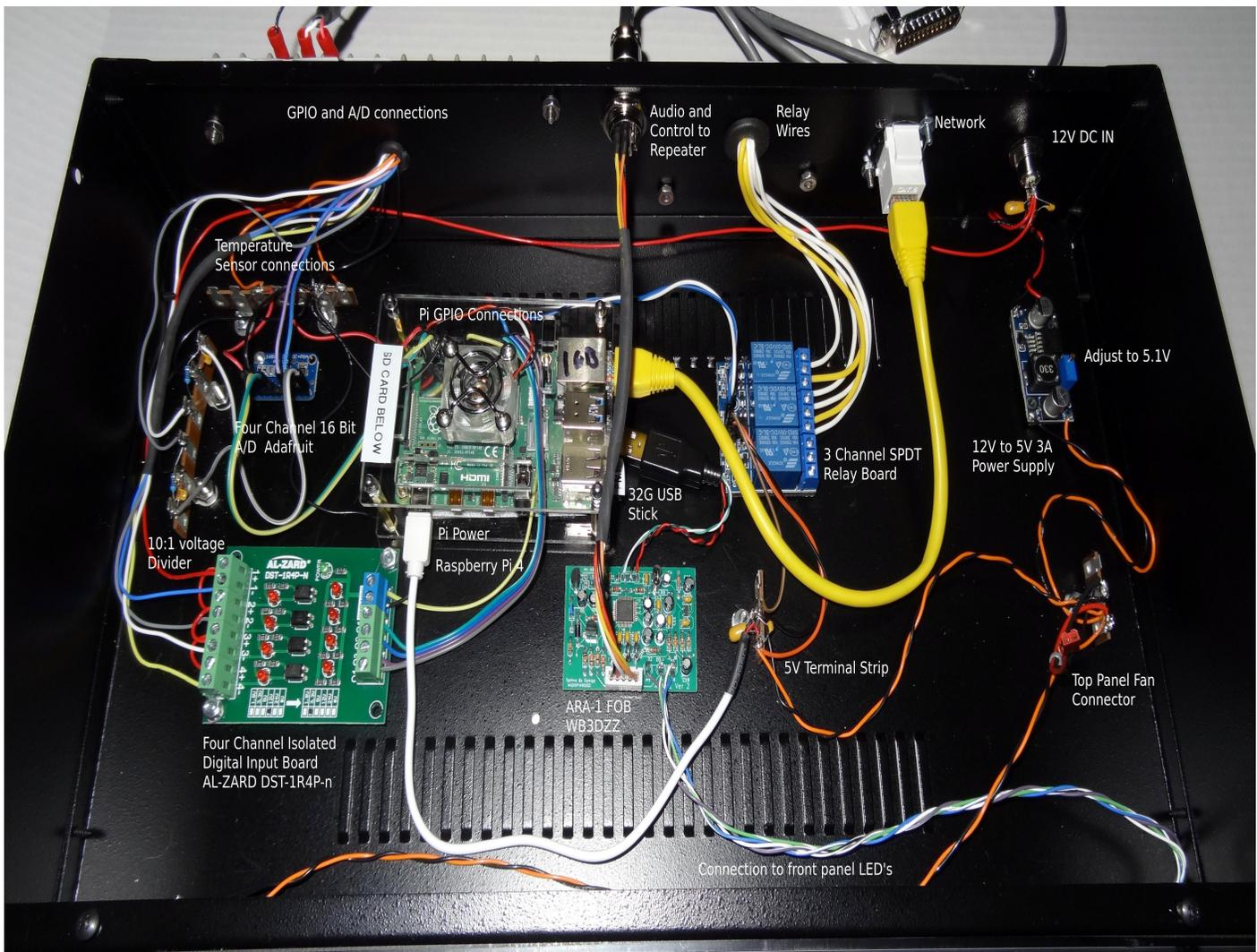
The controller is powered by 12v at the upper right through a barrel connector. This feeds to a 12v to 5V 3A power converter which supplies power for the majority of the components.
