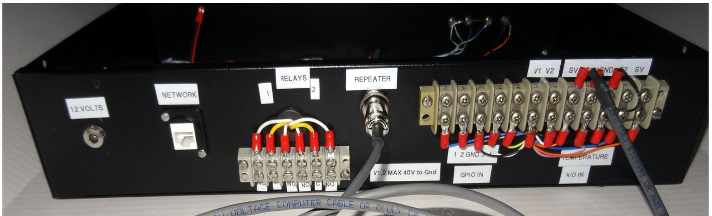
12V power is supplied via a barrel connector shown at the left. Maximum current draw is about 2A
