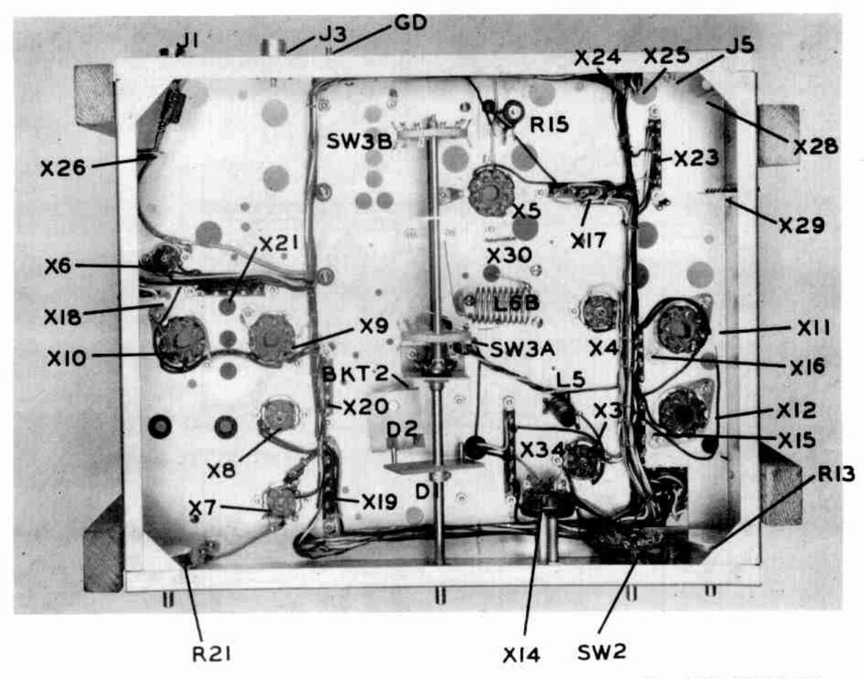
FIGURE 4B. BOTTOM CHASSIS COMPONENT MOUNTING.
