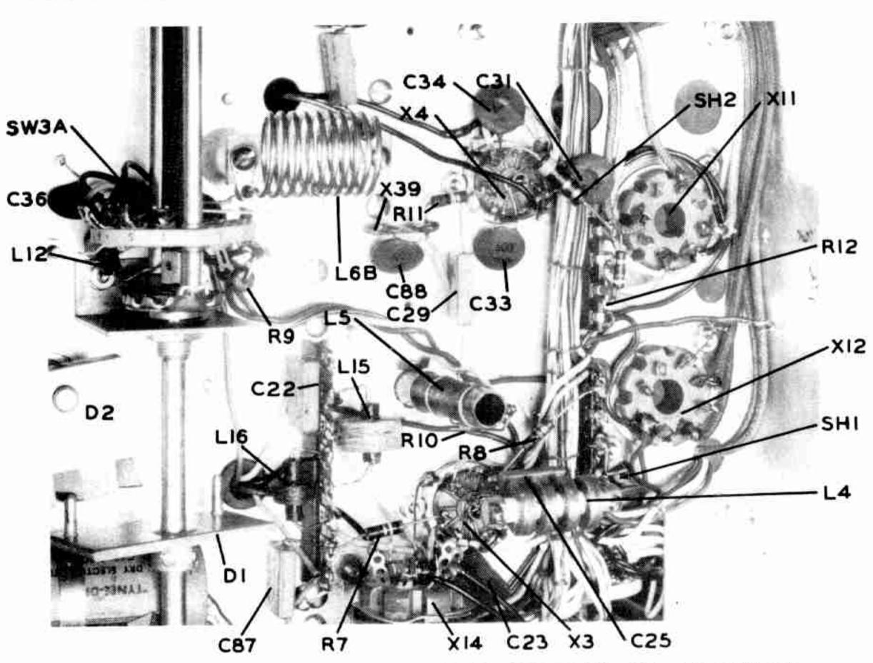
FIGURE 7B. R.F. EXCITER SECTION BOTTOM VIEW.
