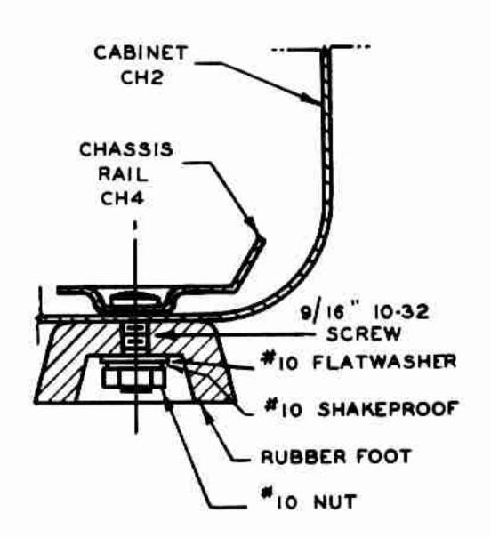
FIG. IOC. CABINET, RAIL, AND FOOT ASSEMBLY
