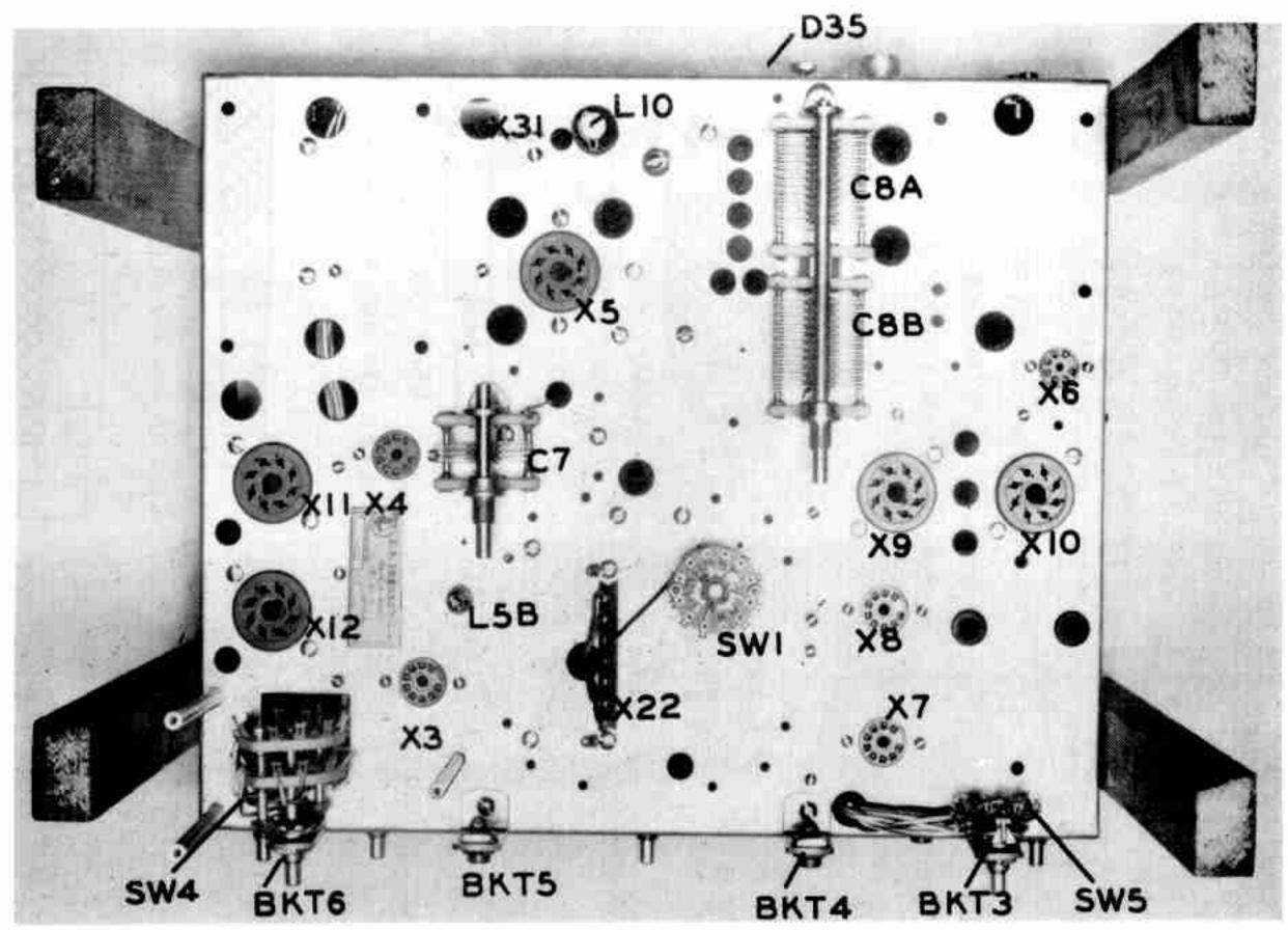
FIGURE 4A. TOP CHASSIS COMPONENT MOUNTING.
