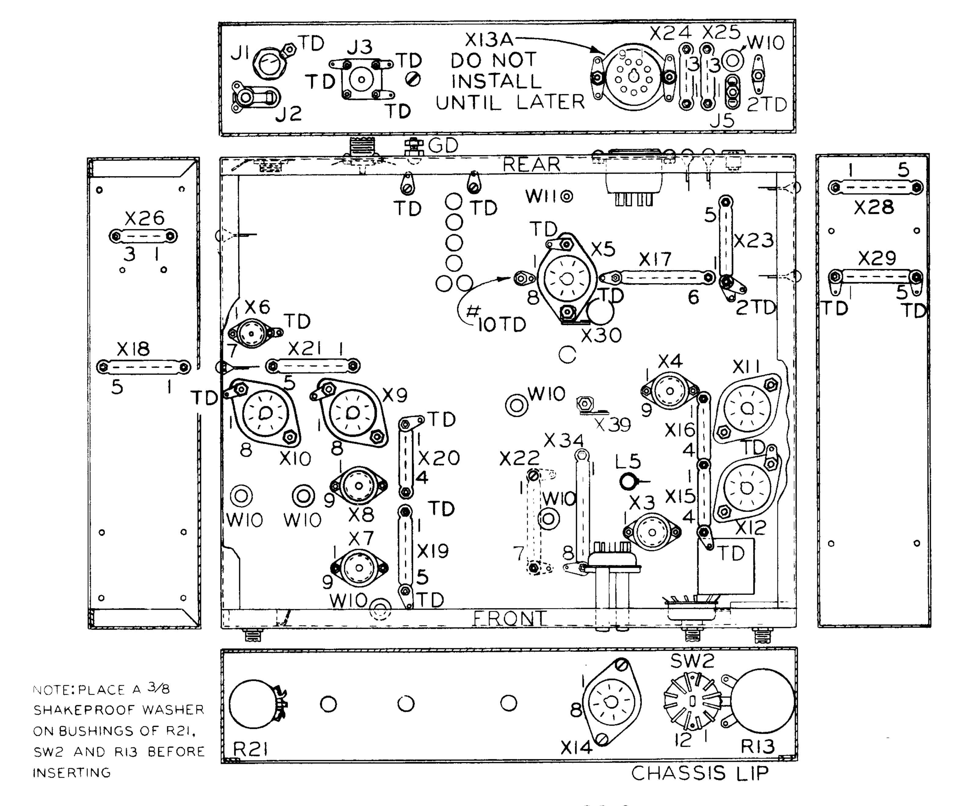
FIG. IA BOTTOM VIEW OF CHASSIS SIDES ARE SHOWN FOLDED OUT ON UNDERSIDE OF CHASSIS
