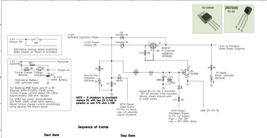
Ignition or Power Switch ON GPIO Power Good Bit High Turn ON Relay or FET with time constant Pi boots Energize Power Shutdown Bit — Pi now holds circuit ON Normal Operation — Pi running
